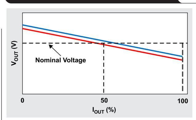
The bigger the  $k$ , the more accurate the current sharing, but the more deviation of output voltage versus load.
