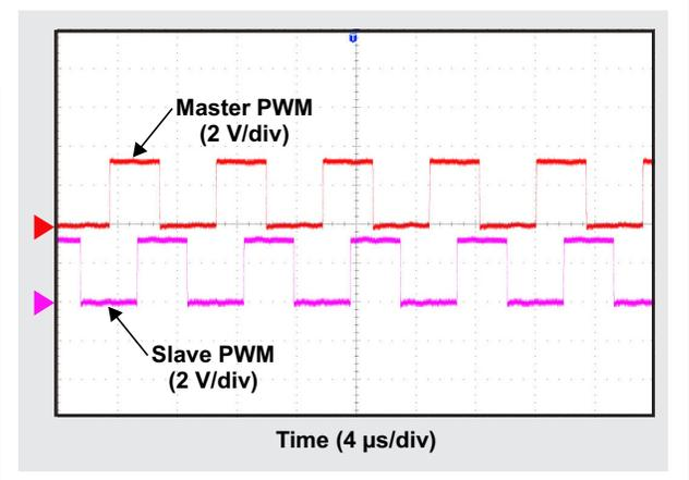
**Figure 3. Master and slave secondary switch-node voltage**
