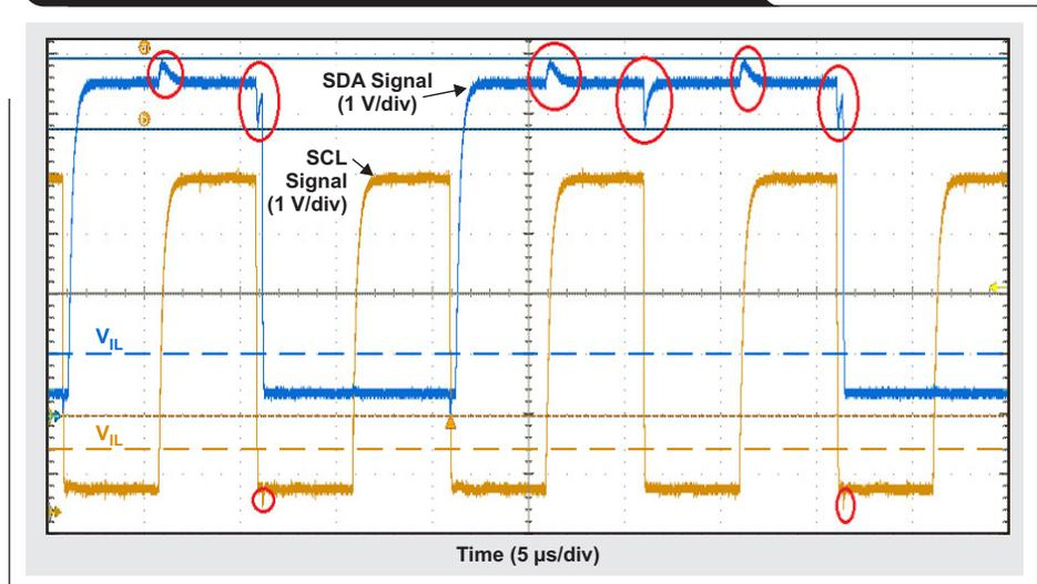
lines as low. Figure 3b shows  $V_{OL}$  higher than  $V_{IL}$  but also lower than  $V_{IH}$ . The SDA/SCL line in Figure 3b is in an unknown state, which is not allowed in I<sup>2</sup>C. The signal may be interpreted by the receiving device as a low or high, depending on the design of the device's input stage.
