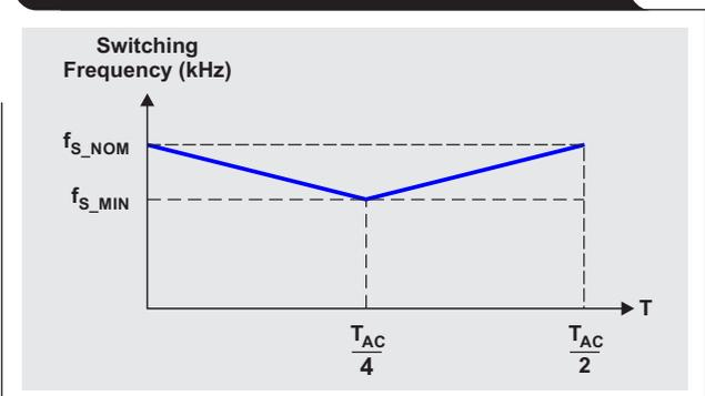
The frequency dithering is not the same as the widely used spread-spectrum frequency dithering technique to reduce electromagnetic interference (EMI) noise. In that technique, the switching frequency is swept back and forth around the nominal value. Because the average switching frequency does not change, the average efficiency is not improved.
