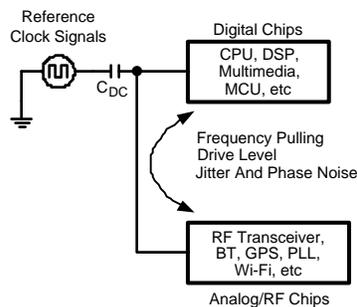
Figure 1. System Function Partitions in Wireless/Portable Electronics
