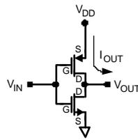
**Figure 4. CMOS Inverter**
