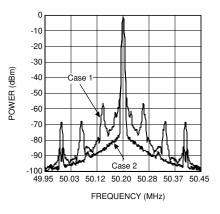
Figure 3-20. Sub-Fractional Spurs (LMX2485E PLL, f<sub>PD</sub> = 2 MHz,2<sup>nd</sup> Order Modulator)
