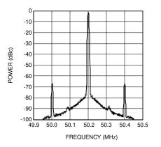
Figure 3-23. LMX2485E Fractional Spurs (Fden = 1/5)
