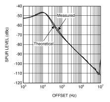
Figure 3-19. Theoretical vs. Measured Data (LMX2485 PLL, Standard Loop Filter, 4<sup>th</sup> Order Modulator
