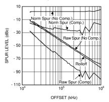
Figure 3-10. Traditional LMX2364 Fractional Spurs
