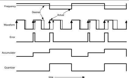
Figure 3-2. Uncompensated Fractional N Example
