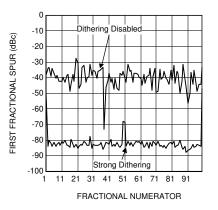
Figure 3-13. Impact of Fractional Numerator (Fraction = x / 101, LMX2485 PLL)
