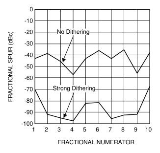
Figure 3-14. Impact of Fractional Numerator (Fraction = x / 11, LMX2485 PLL)
