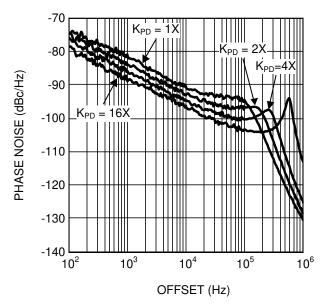
Figure 2-4. Charge Pump Current and 1/f Noise (f<sub>PD</sub> = 50 MHz)
