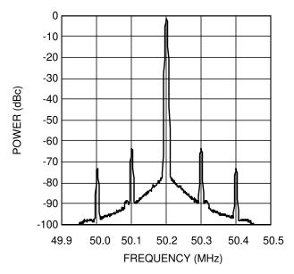
Figure 3-22. LMX2485E Fractional Spurs (Fden = 1/4)
