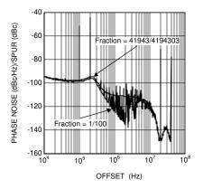
Figure 3-6. Impact of Fractional Denominator (f<sub>PD</sub> = 10 MHz, No Dithering, 3rd Order Modulator)
