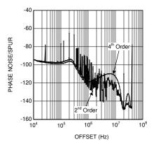
Figure 3-9. Impact of Modulator Order (f<sub>PD</sub> = 10 MHz, No Dithering, Fraction = 1000/1000000)
