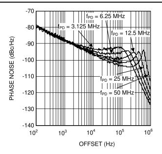
Figure 2-3. 1/f Noise and Phase Detector Frequency (K<sub>PD</sub> = 16X)
