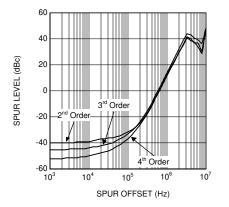
Figure 3-16. Normalized LMX2485 Spurs (BW = 10 kHz)
