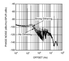
Figure 3-7. Impact of Dithering (f<sub>PD</sub> = 10 MHz, Order = 3<sup>rd</sup>, Fraction = 1/100)
