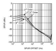
Figure 3-15. Raw LMX2485 Spurs (BW = 10 kHz)
