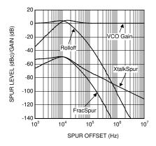
Figure 3-18. Theoretical Spur Decomposition (4<sup>th</sup> Order Modulator)
