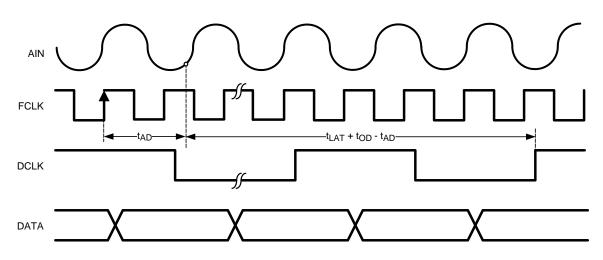
Figure 10. DCLK Generation Timing
