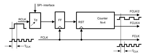
Figure 6. DCLK Generation for Slave Mode
