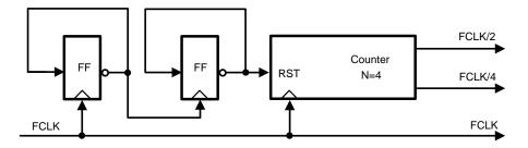
Figure 5. DCLK Generation for Master Mode
