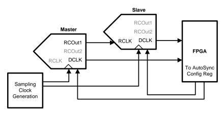
Figure 15. AutoSync Closed Loop Configuration
