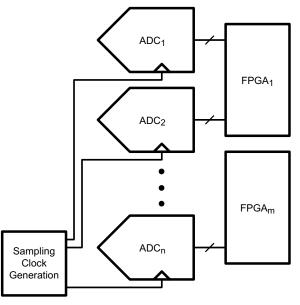
Figure 2. Multiple ADCs in a System
