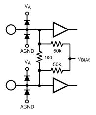
Figure 14. RCLK Equivalent Circuit
