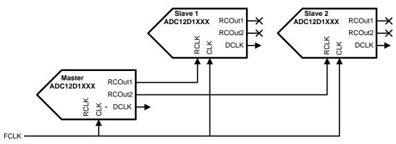
Figure 1. Synchronizing Multiple ADCs Using AutoSync
