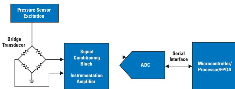
Figure 1. Pressure Sensing System Diagram
