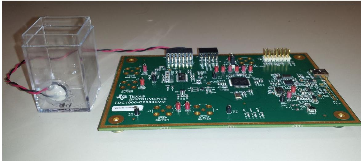
**Figure 2. TDC1000-C2000 EVM with Test Cell**
