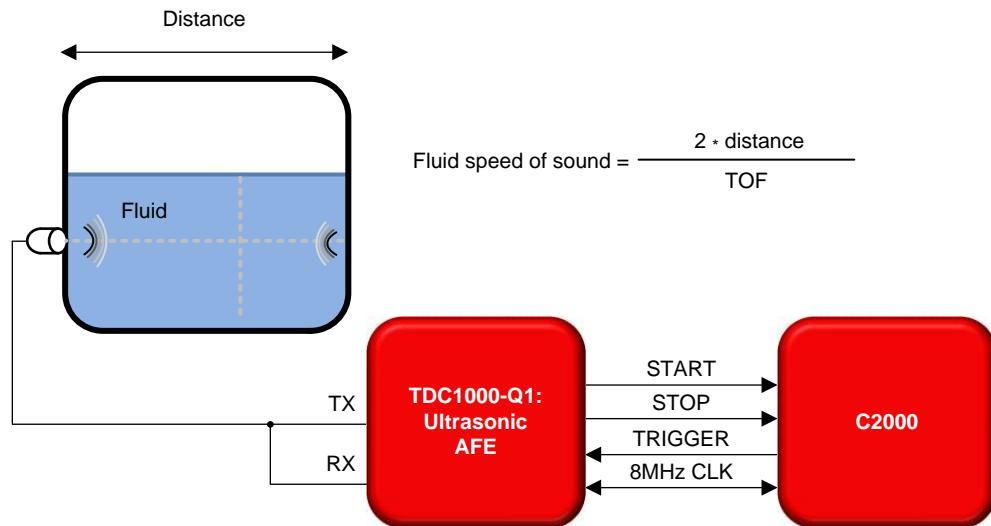
**Figure 1. Fluid Identification Block Diagram**
