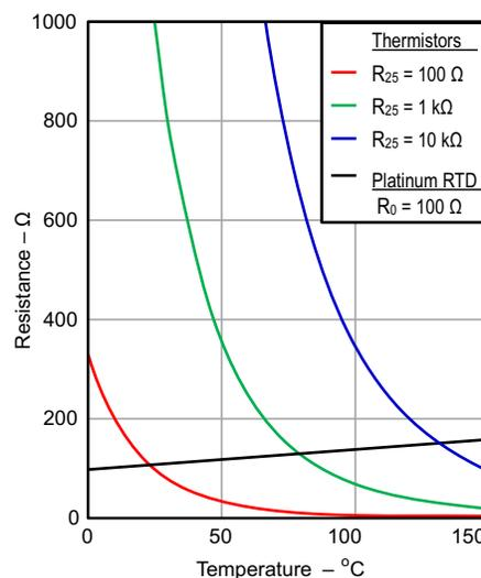
Figure 3. R-T Curve Comparison Between Thermistors and RTD
