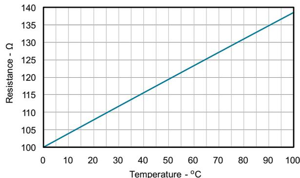
**Figure 1. Resistance – Temperature Curve for PT100**
