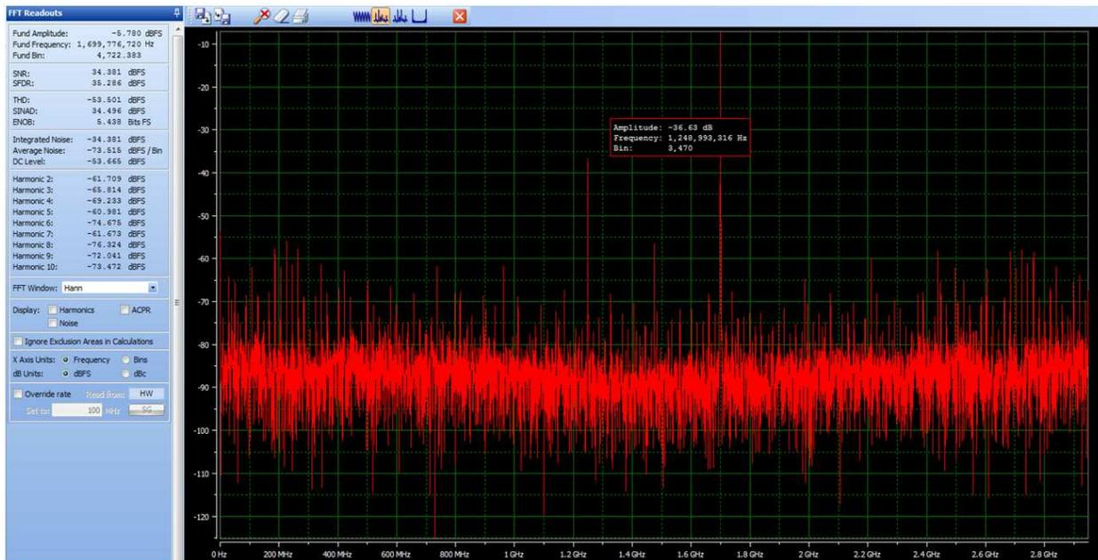
Figure 6. Interleaving Spur at  $F_s/2 - F_{in}$
