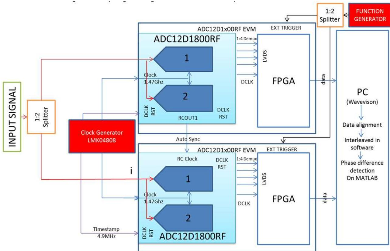
Figure 7. Lab Setup for Interleaving Implementation
