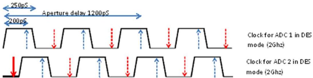
Figure 5. Sampling Timing for Both ADCs
