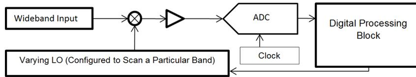
**Figure 3. Wideband Frequency Scanning With Varying LO**
