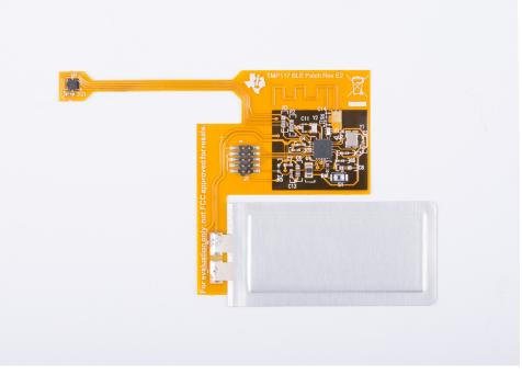
Figure 30. TMP117 BLE Patch Design
