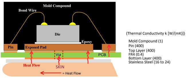
Figure 5. TMP117 Heat Flow Path
