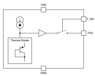
Figure 1. LMT70 Block Diagram
