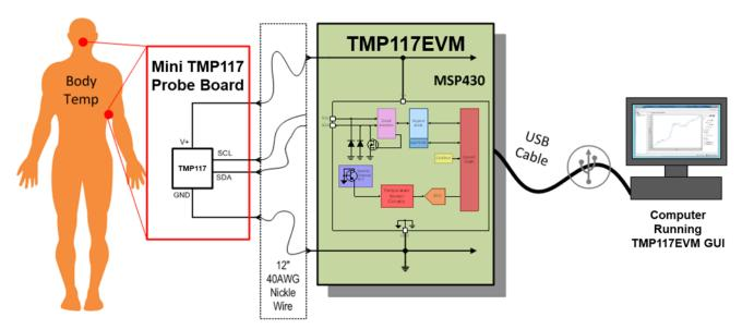
Figure 17. Body Temperature Measurement System
