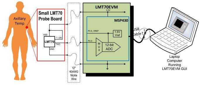
Figure 16. LMT70 Probe Board Thermal Response Measurement System
