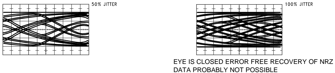
Figure 16. Eye Patterns for NRZ Data Corresponding to Various Peak-to-Peak Transition Jitter
