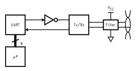
Figure 6. Typical SAE J1708 System Block Diagram
