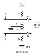
Figure 3. Node Load Circuit
