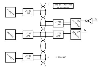
Figure 7. SAE J1708 Typical Bus Configuration and Loading
