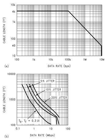
As you increase the cable length, the maximum data rate decreases. The more jitter you can accept, the greater is the allowable data rate for a given length of cable.
