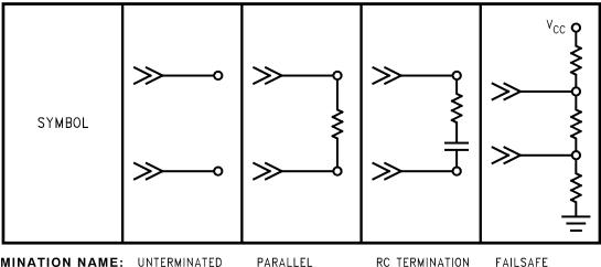
TERMINATION NAME:UNTERMINATEDPARALLELRC TERMINATIONFAILSAFEDATA RATE:LOWHIGHMEDIUMHIGHSIGNAL QUALITY:LIMITEDEXCELLENTLIMITEDEXCELLENTPOWER:LOWHIGHLOWHIGH
