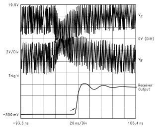
Because of the bus's differentail nature and the receiver's common-mode rejection, the receiver's output (lowest trace) is clean despite large common-mode noise voltages on both of the bus conductors.
