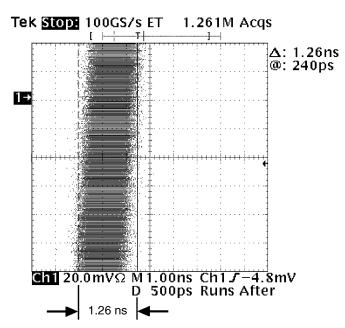
Figure 9. Excessive Jitter Measured at the Jtxout in IEEE 802.3 Gigabit Test Mode 2 on a Compliant GPHY Device
