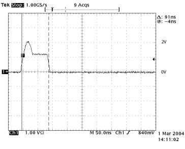
Figure 5. Auto-Negotiation Link Pulse
