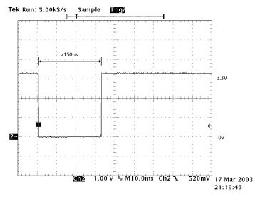
Figure 2. Reset Signal
