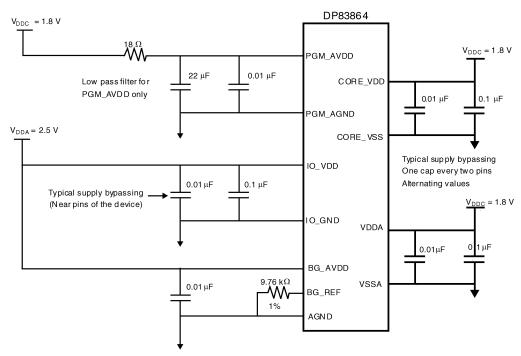
Figure 6. GPHY Power Supplies and Bandgap Voltage
