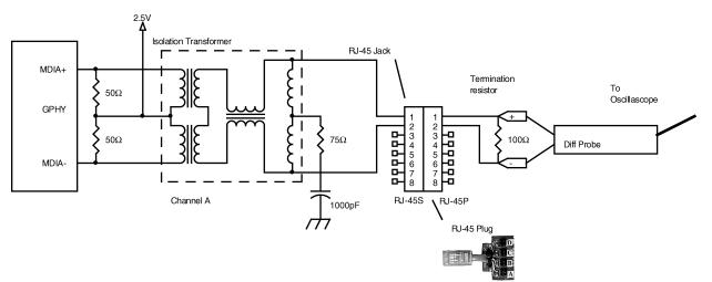
Figure 4. Link Pulse Test On Channel A
