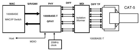
Figure 1. GPHY Block Diagram
