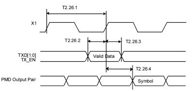
Figure 5. RMII Transmit Timing
