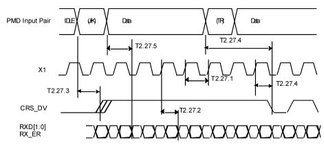
Figure 6. RMII Receive Timing
