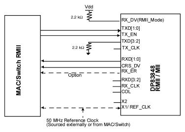
Figure 1. 10/100 Mb/s Twisted Pair Interface
