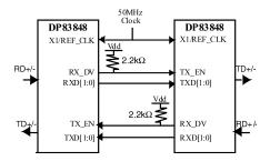
Figure 4. Full-Duplex Extender Connection
