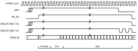
Figure 2. CRS\_DV Generation
