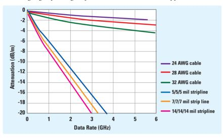
Figure 1. Transmission Media Loss (Differential) Shows the Low Pass Filter Effect
