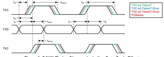
Figure 3. RGMII Timing Diagram Including Duty Cycle Effects
