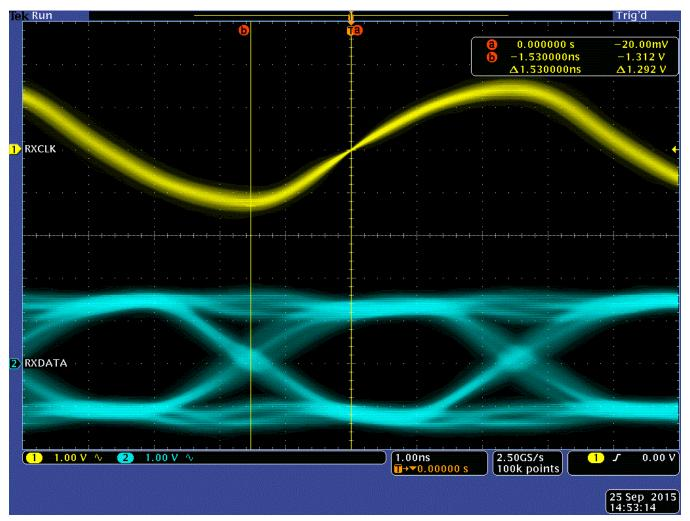
Figure 4. Example Measurement of RGMII Setup Time
