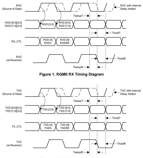
Figure 2. RGMII TX Timing Diagram
