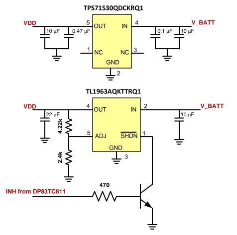
Figure 4. Voltage Supply Schematic for LPSM Implementation
