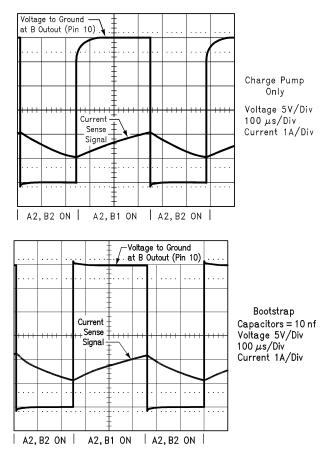
Figure 8. Comparison of Switching Waveforms with and without the Use of Bootstrap Capacitors
