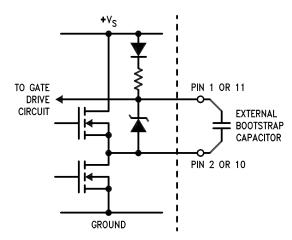
Figure 7. Use of External Bootstrap Capacitors (b)
