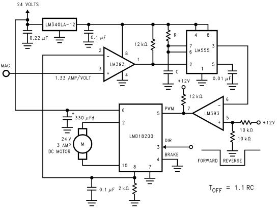
Figure 13. Fixed OFF Time Control
