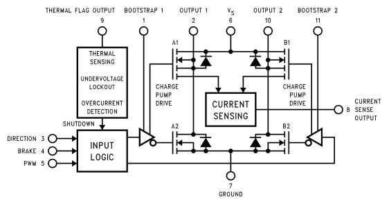
Figure 2. Block Diagram of the LMD18200
