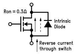
Figure 3. A DMOS Switch with Intrinsic Protection Diode
