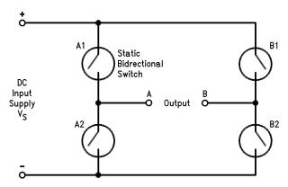
Figure 1. Basic H-Bridge Circuit
