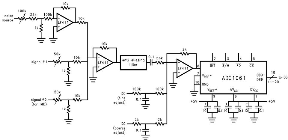
FIGURE 8. Setup for Investigating the Effects of Dither
