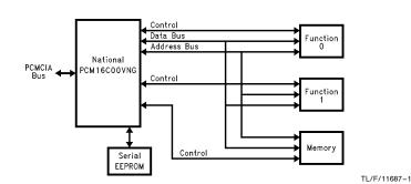
FIGURE 1. Block Diagram of a Multi-Function PC Card Using the National® PCM16C00VNG
