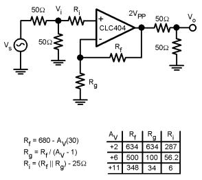
Figure 5. Test Circuit and Table of Values
