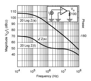
Figure 2. Feedback Transimpedance
