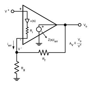
Figure 1. Current Feedback Amplifier Internal Elements
