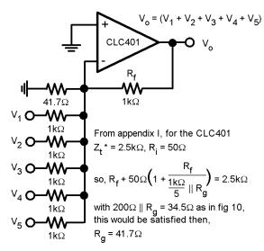
Figure 10. Loop Gain Adjusted in Inverting Summing Application
