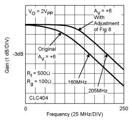
Figure 8. Frequency Response With Loop Gain Response
