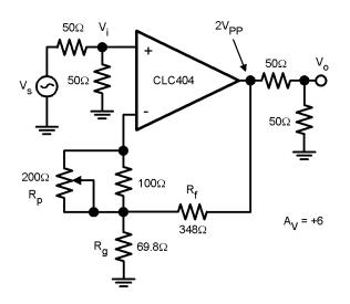
Figure 7. Adjustable Frequency Response
