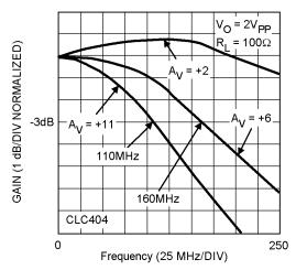
Figure 3. Frequency Response vs. Gain for  $R_{\rm f}$  Fixed = 500 $\Omega$
