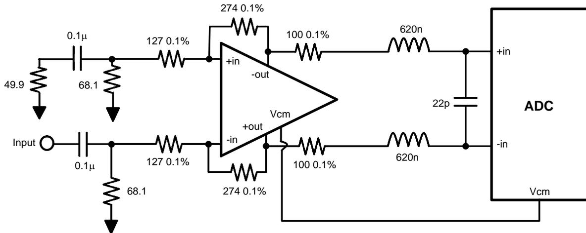
Figure 2. LMH6552 Driving a Circuit With 2<sup>nd</sup> Order Low Pass Filter
