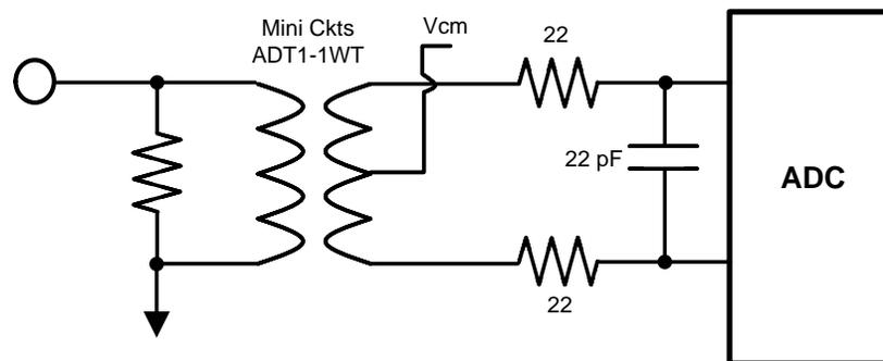
**Figure 1. Transformer Drive Circuit**
