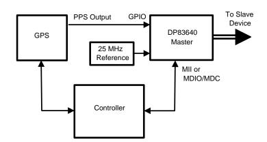
Figure 1. Block Diagram Using 25 MHz Reference not Cconnected to the GPS sSurce
