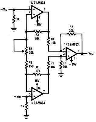
R<sub>1</sub>, R<sub>2</sub>, and R<sub>3</sub> are 0.1% tolerance units (or R<sub>2</sub> can be trimmed).
