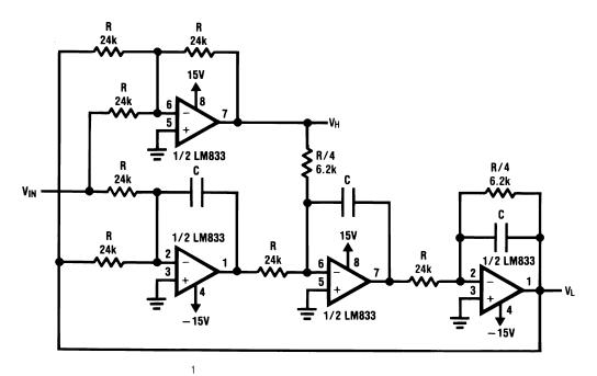
The crossover frequency is equal to  $\overline{2\pi RC}$
