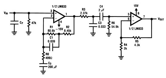
Figure 3. Two-Amplifier RIAA Phono Preamplifier with Very Accurate RIAA Response
