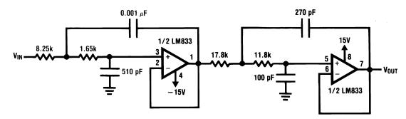
The filter gain is down 3 dB at about 40 kHz. As with the infrasonic filter, 1% tolerance components should be used for accurate response.
