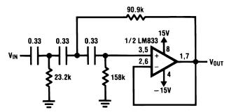
Filter characteristic is third-order Butterworth with −3 dB frequency at 15 Hz. Resistor and capacitor values shown are for 1% tolerance components. 5% tolerance units can be substituted in less critical applications.
