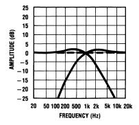
For the circuit of Figure 9, a<sub>1</sub>=4, a<sub>2</sub>=4, and a<sub>3</sub>=1. Note that the summed response (dashed lines) is perfectly flat.
