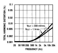
The lower curve is for an output level of 300mVrms and the upper curve is for an output level of 1Vrms.
