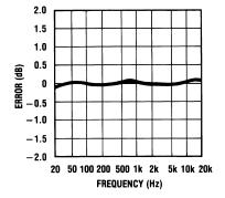
The maximum observed error for the prototype was 0.1 dB.
