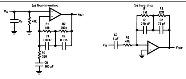
Figure 2. Two Typical Operational Amplifier-based Phonograph Preamplifier Circuits
