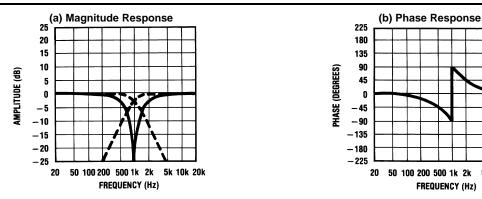
The individual high-pass and low-pass outputs are superimposed (dashed lines).
