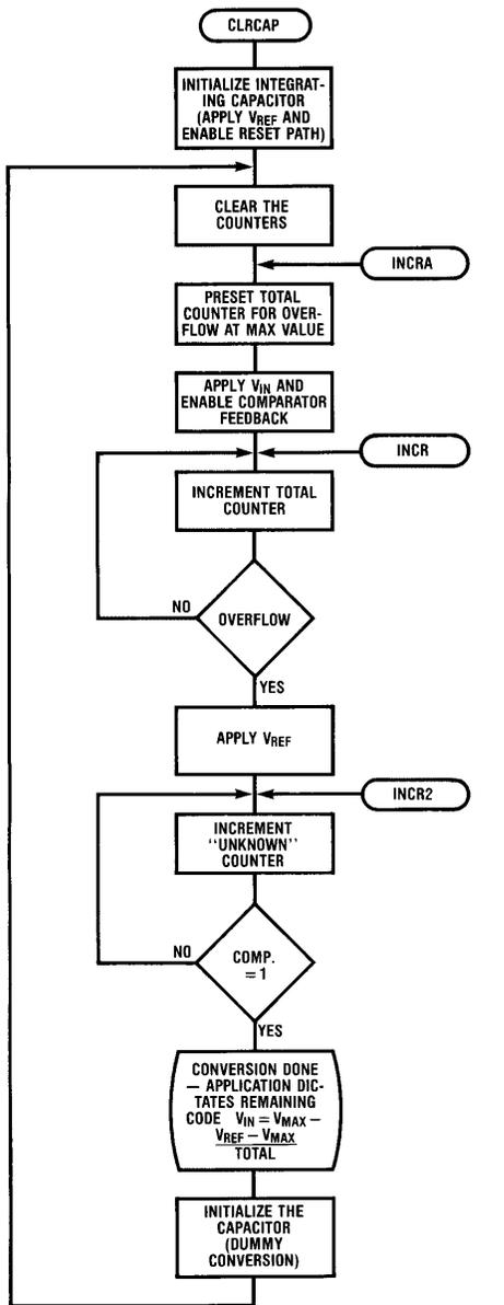
FIGURE 17B. Modified Dual Slope Flow Chart
