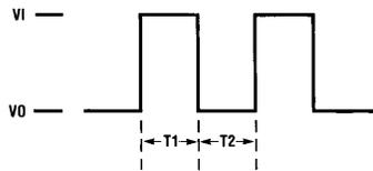
$$V_C = \frac{(V_1 - V_0) \times T_1}{T_1 + T_2}$$
