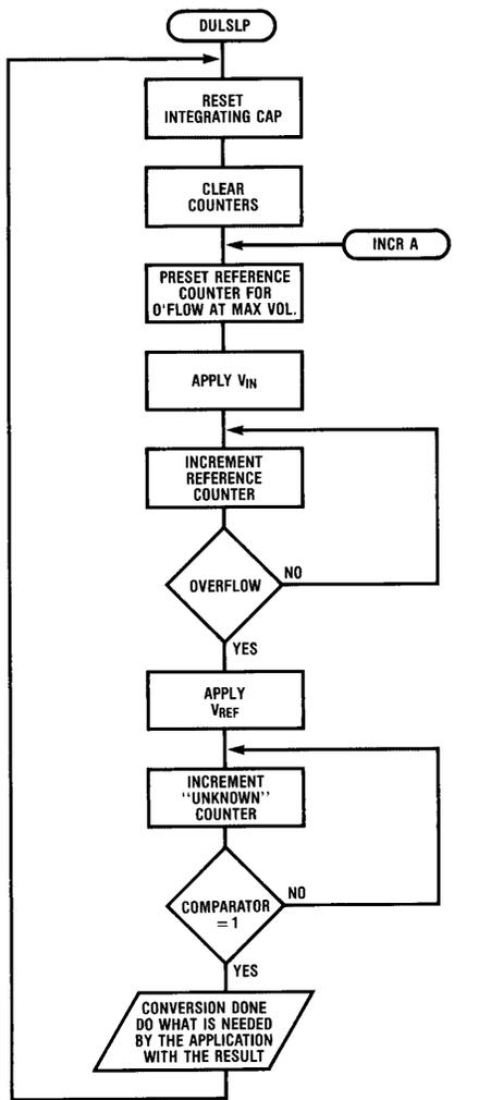
FIGURE 14B. Basic Dual Slope A/D Flow Chart
