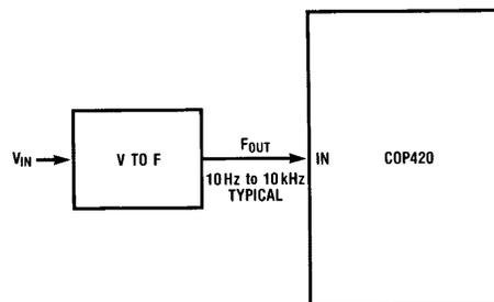
FIGURE 18. V to F Converter — Basic Concept
