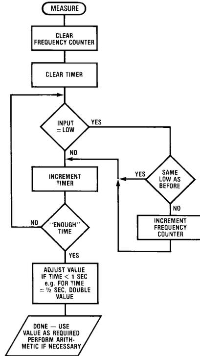
FIGURE 19B. V to F by Counting Pulses
