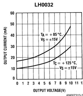
**FIGURE 21. Continuous Output Drive Capability**
