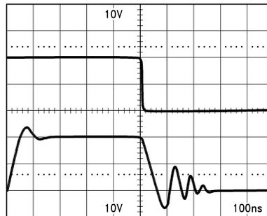
FIGURE 17. LH0032 Unity Gain Non-Inverting Large Signal Pulse Response: T<sub>A</sub> = 25°C, C<sub>C</sub> = 10 pF, C<sub>A</sub> = 100 pF
