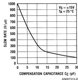
FIGURE 25. LH0032 Slew Rate vs. Frequency Compensation Capacitance
