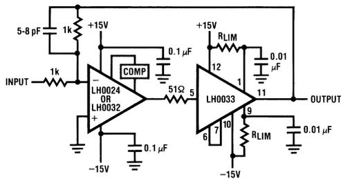
FIGURE 6. Wide Band Amplifier with 100 mA Output Capability
