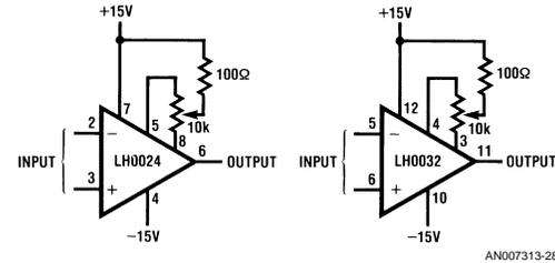
FIGURE 24. Offset Voltage Adjustment
