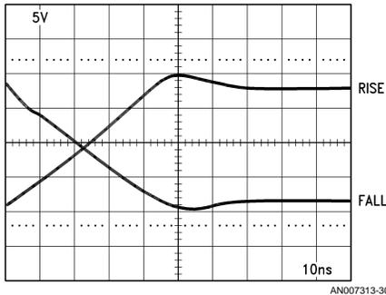
**FIGURE 26. LH0024 Slew Response, Unity Gain Inverting Mode**
