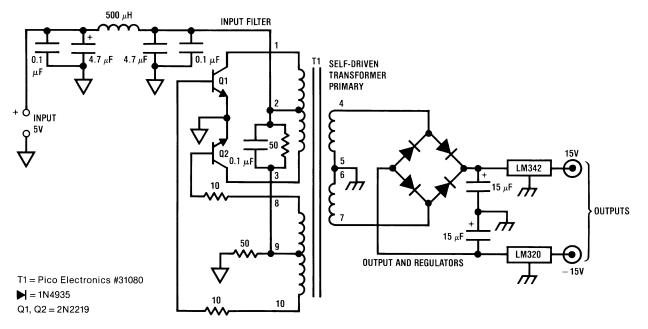
Figure 1. Typical DC-DC Converter
