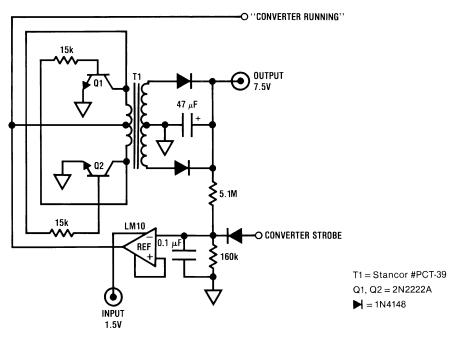
Figure 9. Low Power Converter
