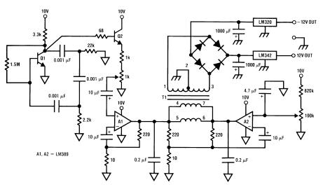
Figure 7. Sine Wave Driven Converter
