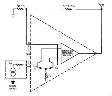
$V_{OUT} \cong (n+1) \ V_{IN} + V_{OS} \times (n+1) + (I_{b2} - I_{b1}) \times r_s \times (n+1) + V_{noise} \times (n+1) + I_{noise} \times (r_s + R_{IN}) \times (n+1)$
