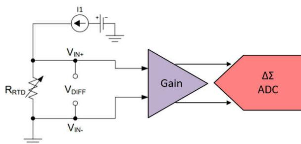
Figure 1. Simplified RTD Circuit
