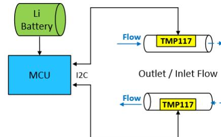
**Figure 5. Heat and Cold Meter With TMP117 Block Diagram**
