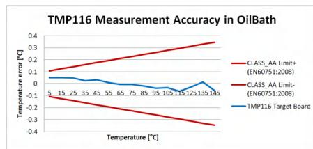
**Figure 4. TMP116 Target Board Meets Class AA Limits Without Calibration**
