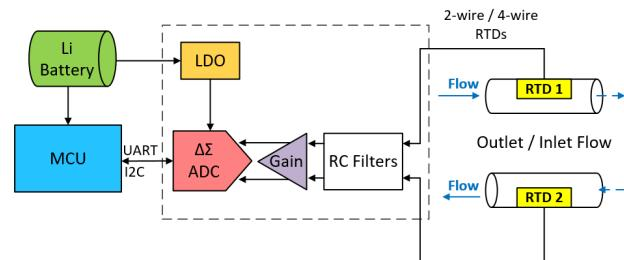
Figure 2. Heat and Cold Meter With RTD Block Diagram
