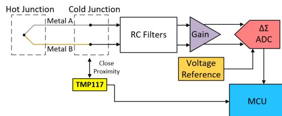
**Figure 6. Cold Junction Compensation With TMP117 Block Diagram**
