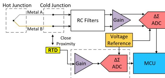
**Figure 3. Cold Junction Compensation With RTD Block Diagram**
