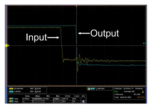
Figure 2-8. Propagation Delay High to Low
