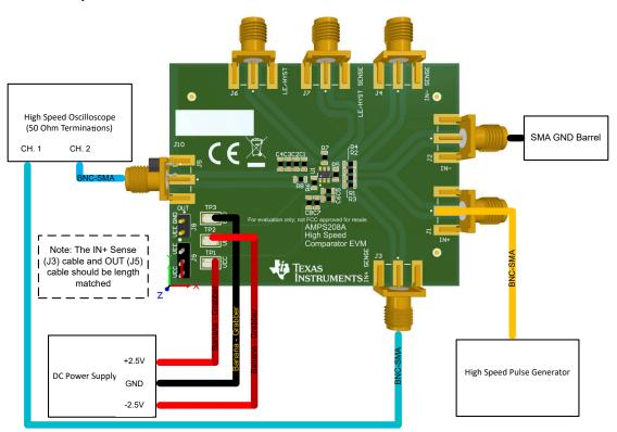
Figure 2-6. HS-COMPARATOR-EVM Quick Start Setup Using TLV1H103
