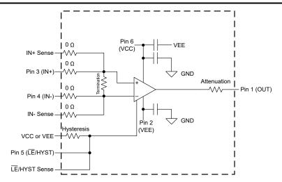
Figure 1-3. EVM Pin Assignments for Evaluating 6-pin Devices
