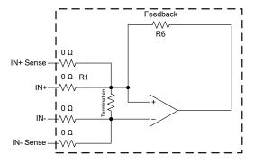
Figure 2-4. External Hysteresis Schematic
