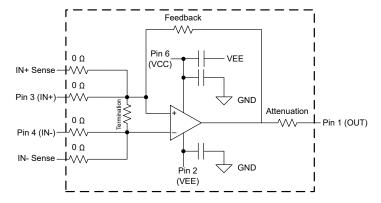
Figure 1-2. EVM Pin Assignments for Evaluating 5-pin Devices
