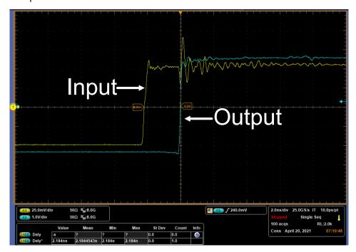
Figure 2-7. Propagation Delay Low to High
