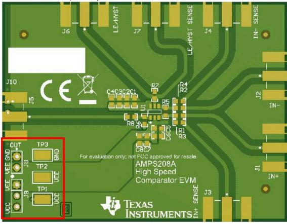
Figure 2-1. Power Supplies Connection
