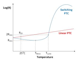
Figure 2. Comparison Between Linear Versus Switching PTC Thermistors
