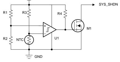
Figure 4. Thermal Switch Circuit
