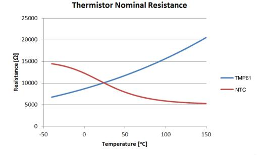
Figure 10. Resistance Versus Temperature Profile of a Linearized NTC Compared to TMP61
