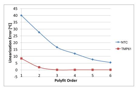
Figure 7. Linearization Error Versus Polyfit Order
