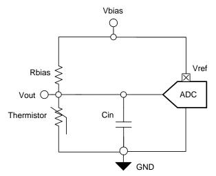
Figure 5. Ratiometric Temperature Monitor Circuit
