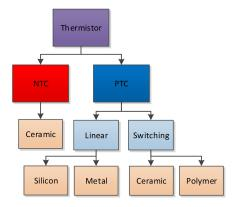
Figure 1. Generalized Thermistor Family Tree
