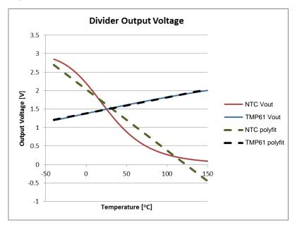
Figure 6. Example Voltage Divider Output and 1<sup>st</sup> Order Polyfit Linearization
