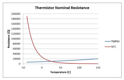
Figure 3. Resistance Verus Temperature Profile of NTC and TMP61
