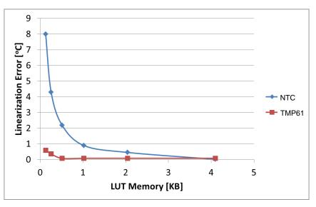
Figure 8. Linearization Error Versus LUT Memory
