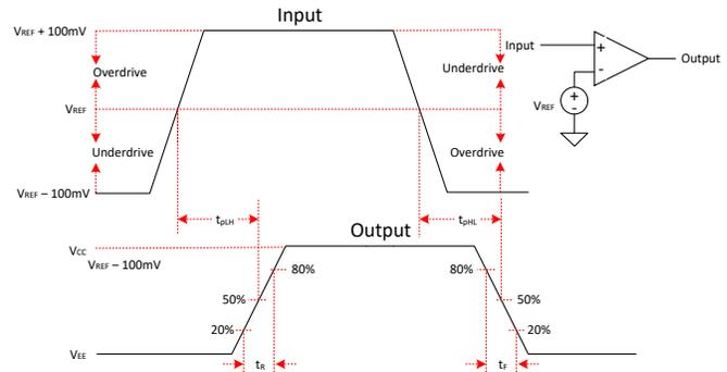
Figure 4. AC Timing Response
