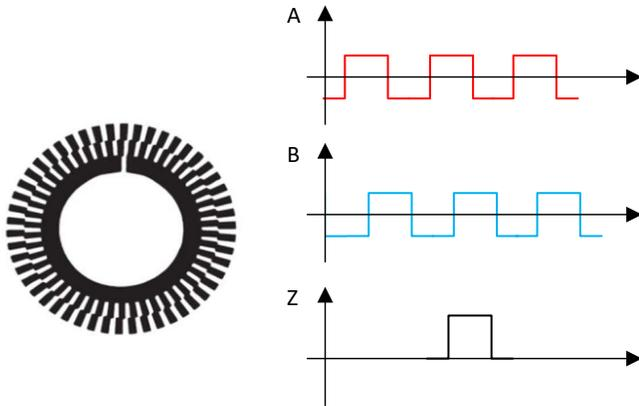
**Figure 5. Zero-Reference Signal**
