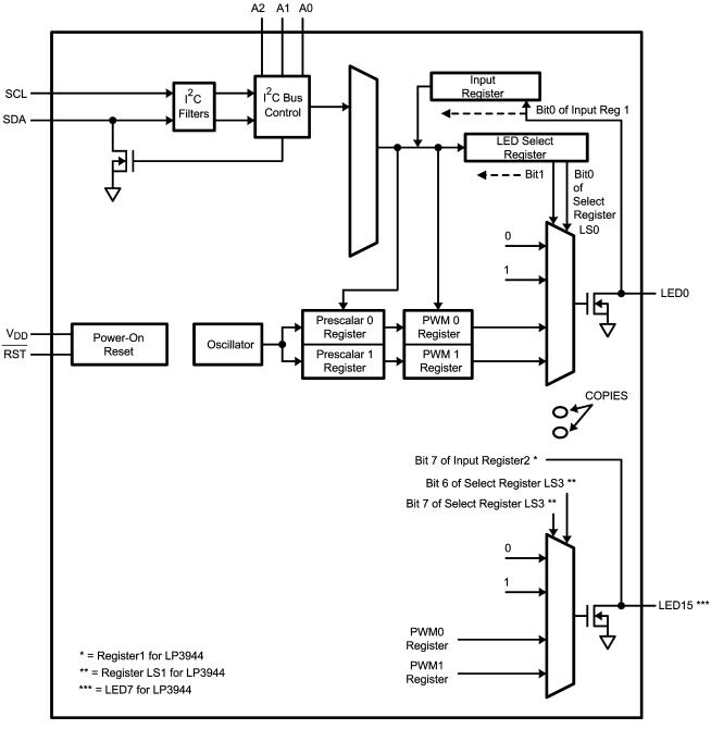
Figure 2. LP3943/44 Block Diagram
