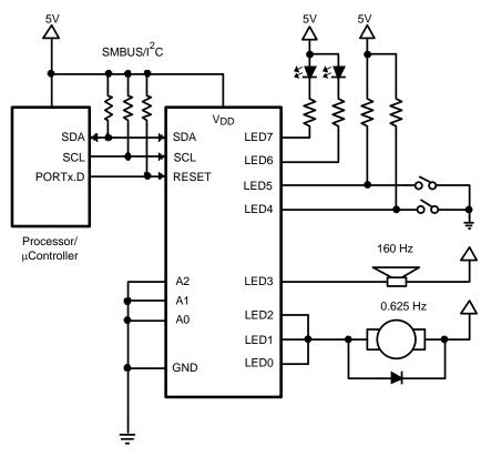
Figure 3. LP3944 in Mixed Mode Configuration
