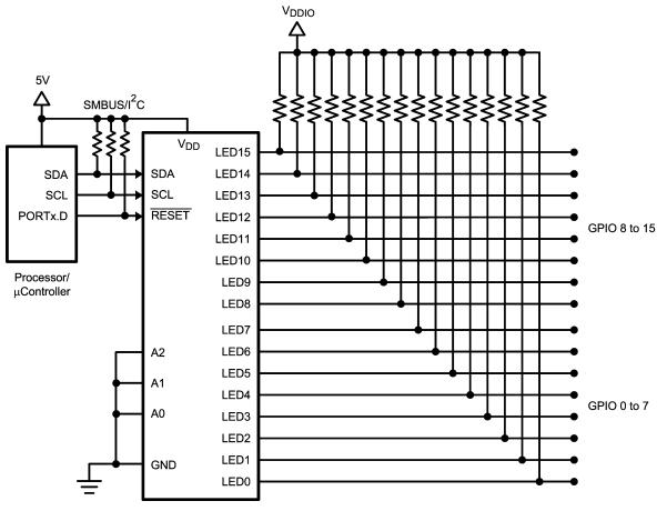
Figure 1. LP3943 Configured to 16 Channel GPIO Expander
