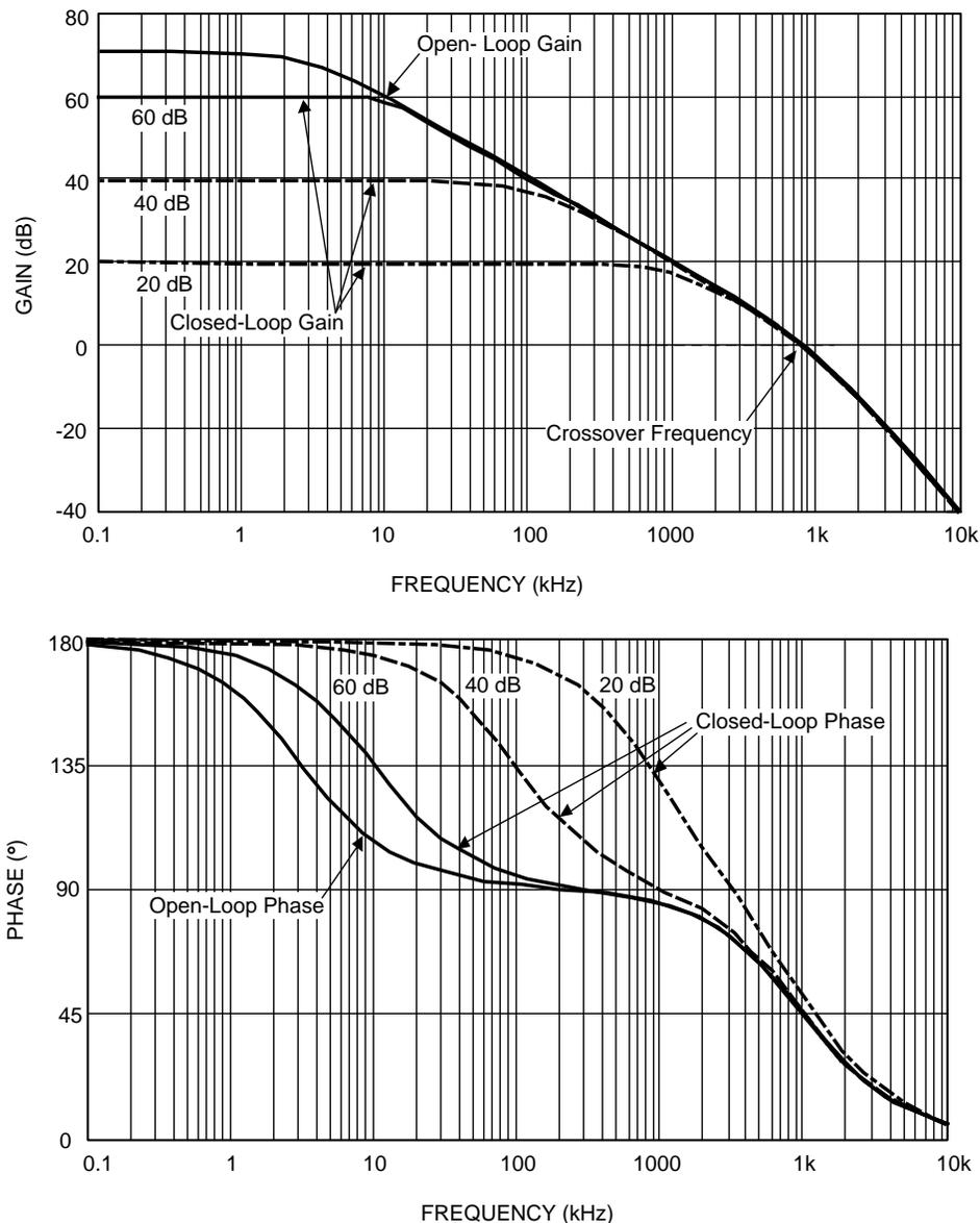
**Figure 3. (a) Gain and (b) Phase versus Frequency Curves of the Open-Loop and Closed-Loop EA**
