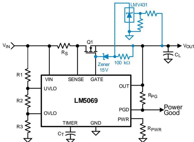
Figure 7. Accurate Output Voltage Clamp Circuit
