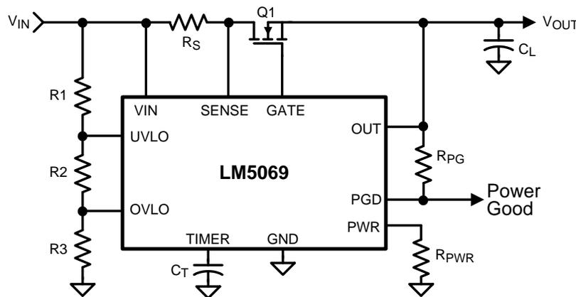
Figure 1. LM5069 Basic Application Circuit
