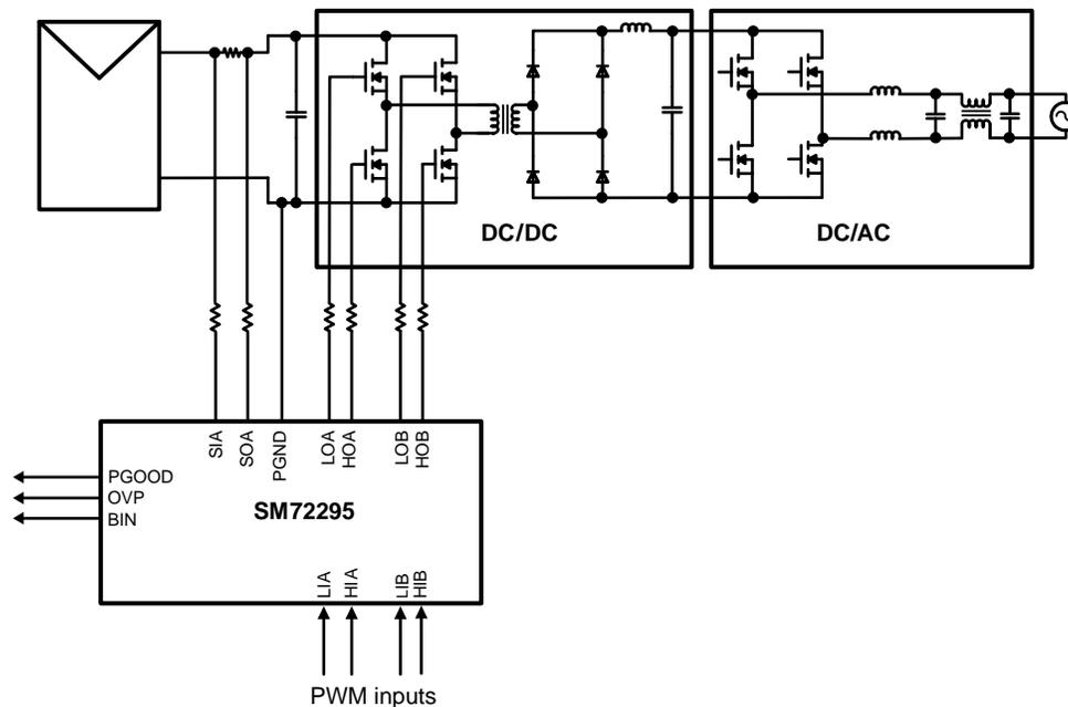
The DC/DC stage is implemented as a voltage-fed full-bridge converter, and the DC/AC stage is implemented as a MOSFET Full-bridge.
