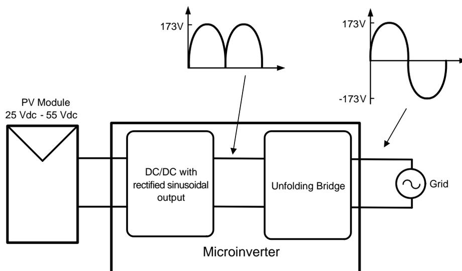
The DC/DC stage can be implemented as a quasi-resonant interleaved flyback or another topology.
