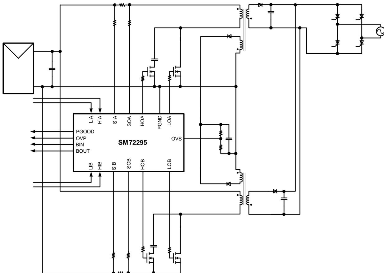
Current sensing is implemented with high-side current sense resistors, and output overvoltage shutdown is implemented using voltage sense windings and the OVS pin.
