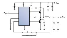
Figure 2: Synchronous PWM Switcher Topology
