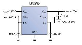
Figure 3: LP2995 Typical Application Circuit
