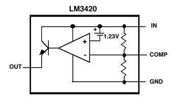
FIGURE 9. BLOCK DIAGRAM OF LM3420
