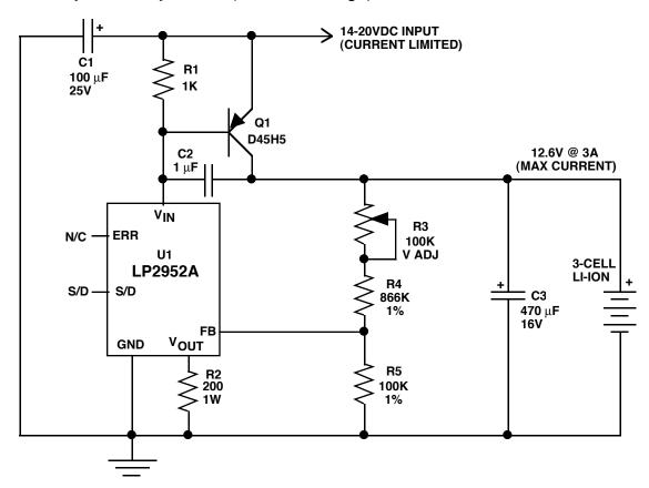
FIGURE 8. 3-CELL, 3A CHARGER USING THE LP2952
