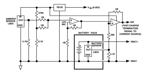
FIGURE 3. AT DETECTOR CIRCUIT
