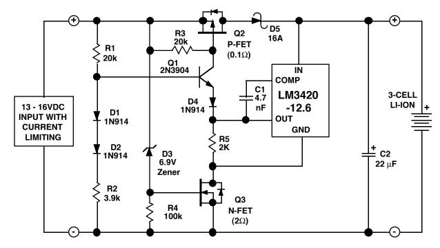
FIGURE 10. 3-CELL, 3A CHARGER USING THE LM3420
