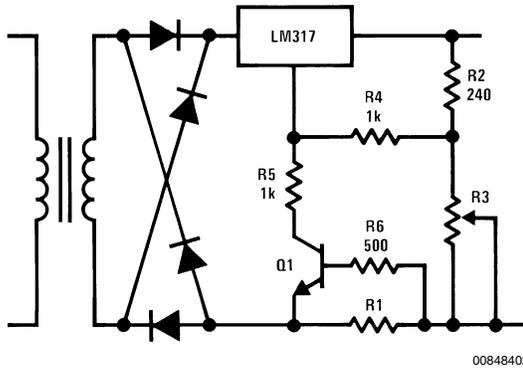
**FIGURE 2. Constant Voltage Charger with Peak Current Limiting**
