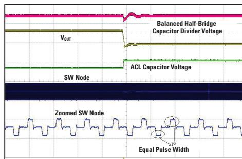
**Figure 5. Balanced Half-Bridge Capacitor Waveform in a Soft-Short Condition Employing Average Current Limit**
