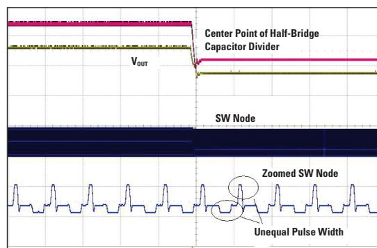
**Figure 2. Current Limit Waveforms of Half-Bridge Topology Employing Peak Cycle-by-Cycle Current Limit**
