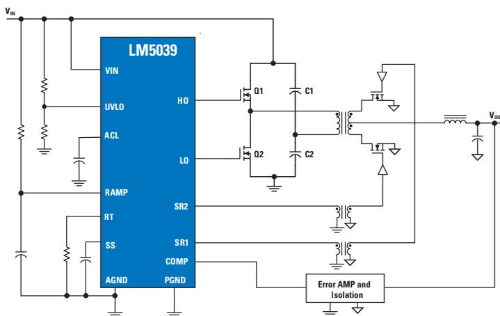
Figure 1. Simplified Schematic of a Half-Bridge Topology
