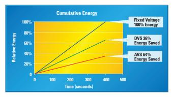
Figure 1. Energy Savings with DVS and AVS
