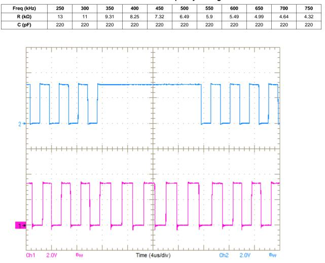
Figure 2. Sync Clock and 555 Timer Output Pulses
