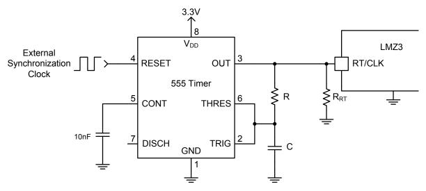
Figure 1. 555 Timer Uninterruptible Clock Circuit
