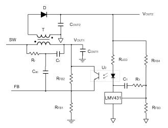
Figure 3. Optocoupler for Secondary Output Signal Transmission
