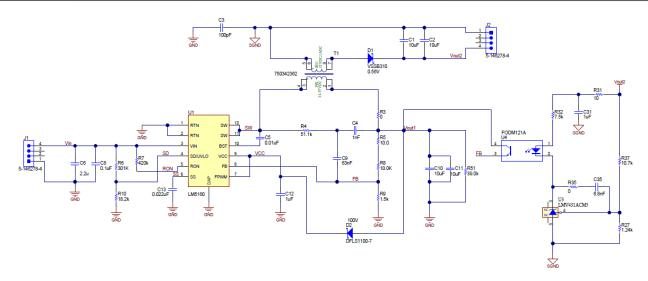
Figure 5. LM5160 Flybuck With Optocoupler Schematic
