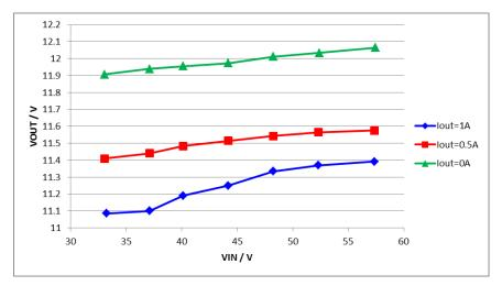
Figure 8. Input Regulation: LM5160 Flybuck Without Optocoupler
