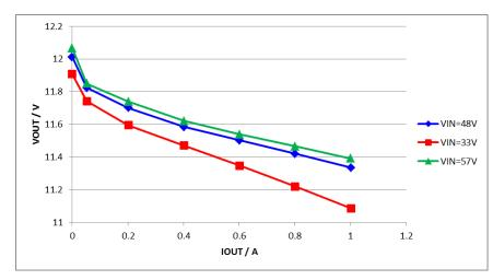
Figure 6. Load Regulation: LM5160 Flybuck Without Optocoupler
