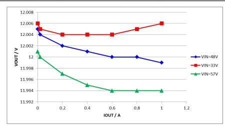
Figure 7. Load Regulation: LM5160 Flybuck With Optocoupler
