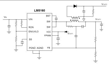
Figure 1. LM5160 Flybuck Solution
