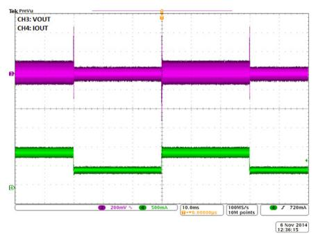
Figure 12. Transient Test ( $V_{IN}$  = 48 V,  $V_{OUT2}$  = 12 V,  $I_{OUT2}$  = 0.5 A to 1 A, 0.1 A/µs Slew Rate)
