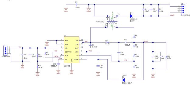
Figure 2. LM5160 Flybuck Schematic
