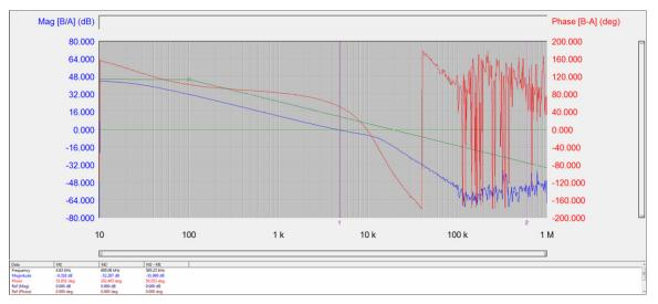
Figure 4. Loop Test Result With Type I Compensation Network
