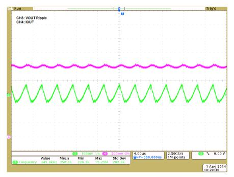
Figure 11. Output Voltage Ripple ( $V_{IN}$  = 48 V,  $V_{OUT2}$  = 12 V,  $I_{OUT2}$  = 1 A)
