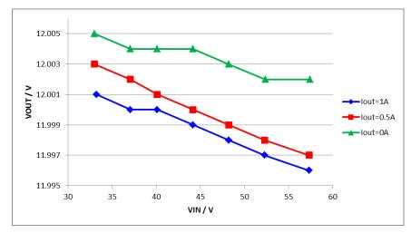
Figure 9. Input Regulation: LM5160 Flybuck With Optocoupler
