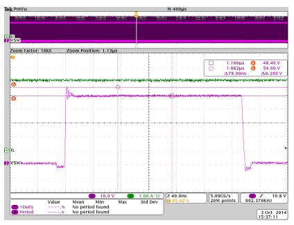
Figure 10. Switch Node Waveforms
