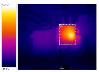
Figure 11. With No Airflow, 2-W Dissipation
