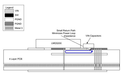
Figure 3. Cross-Section of the LMG5200 PCB Layout
