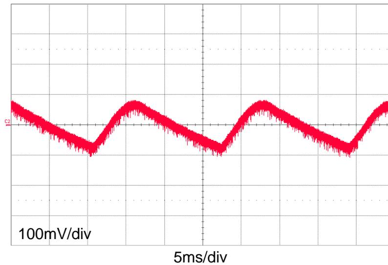
Figure 3. Voltage Ripple at  $V_{DC}$
