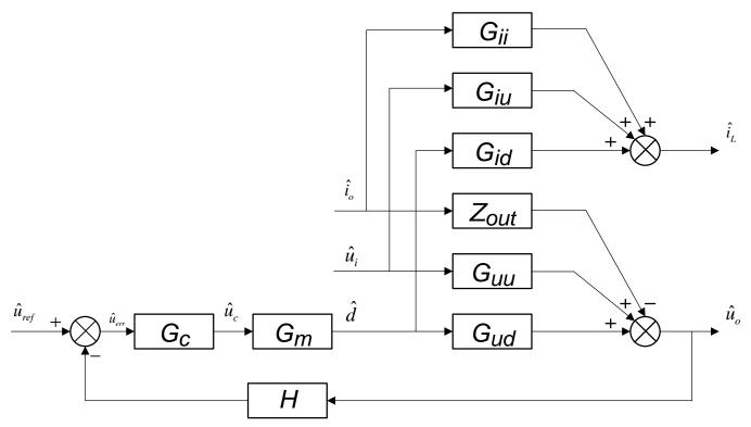
Figure 4. VMC Closed Loop Buck Controller Block Diagram
