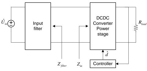
Figure 8. Buck Control Block Diagram With LC Filter
