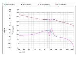
Figure 10. Simplis Simulation Loop Gain
