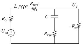
Figure 18. Equivalent Circuit for Stability Analysis
