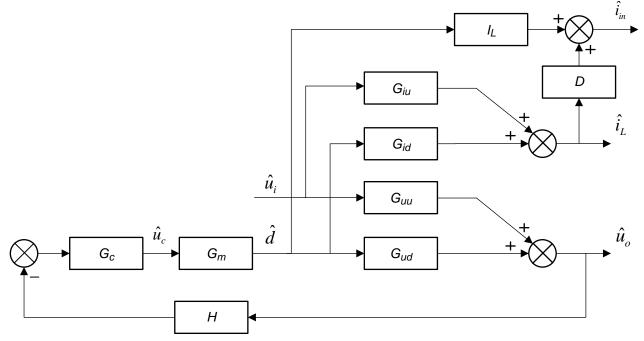
Figure 11. Closed Loop Input Impedance Calculation Block Diagram
