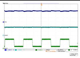
Figure 21. Load Transient Test on EVM
