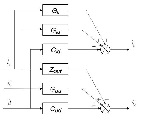
Figure 3. Open-Loop Buck Controller Block Diagram
