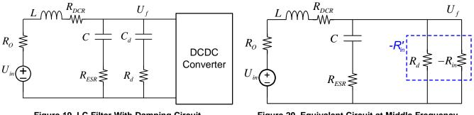
Figure 19. LC Filter With Damping Circuit
