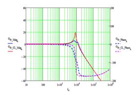
Figure 15. Input Filter Frequency Response With Closed Loop
