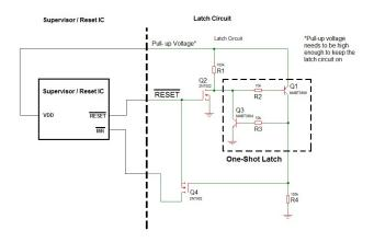
Figure 3. Voltage Supervisor Latch Circuit
