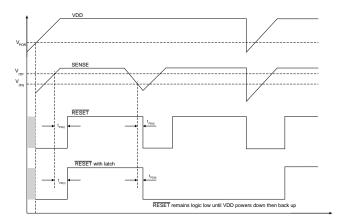
Figure 4. Normal vs Latched Operation Timing Diagram
