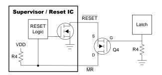
Figure 2. Voltage Supervisor Operation with Latch
