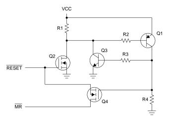
Figure 1. External Latch Circuitry
