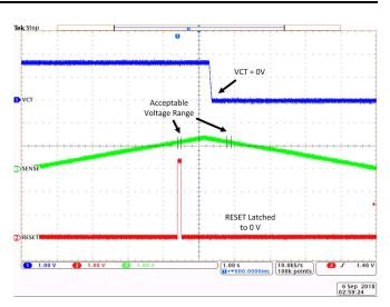
Figure 6. Fault Causing Latching Functionality
