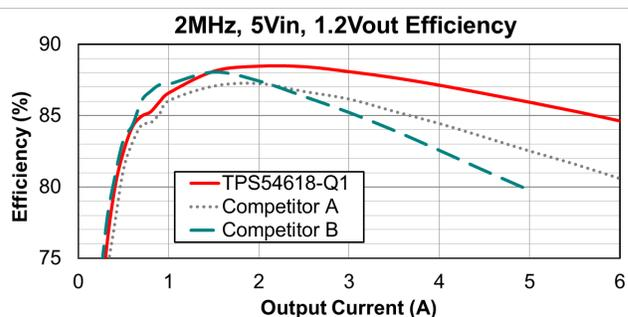
Figure 1. Efficiency of TPS54618-Q1 vs competitors' devices
